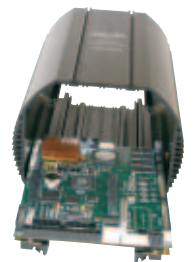
Hercules CPU mounted on ACC-VT-EBX in Versa-Tainer
