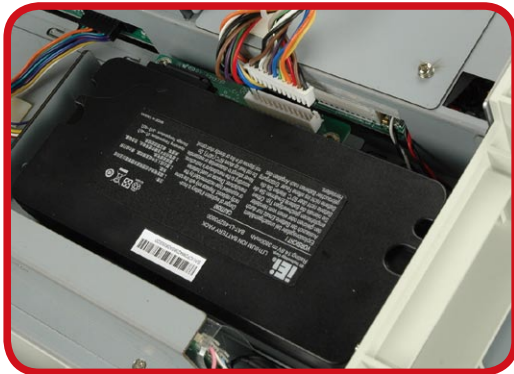
Battery -Type: Li-Ion 4S2P -Normal Voltage: 14.8V, 3800mAH -Backup: 100W/10min
