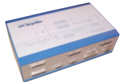
OEM-PIP assembled with up to 4 additional PC/104 cards
